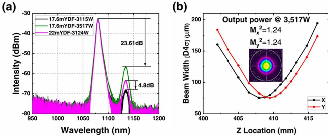
**Figure 5.** Experimental results of bidirectional pumping after shortening the active fiber of the amplifying section: (a) spectral comparison before and after the shortening of the fiber; (b) result of the beam quality  $M^2$  factor at the power of 3517 W. Inset: a beam profile of the output laser.
