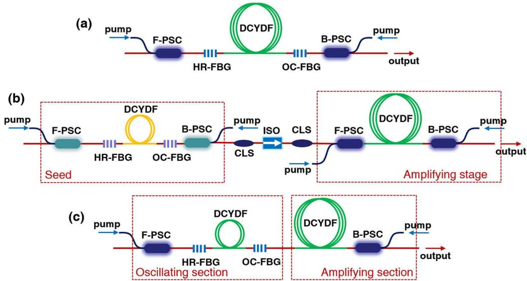
**Figure 1.** Schematic diagram of the three structures of fiber lasers: (a) fiber laser oscillator based on the FP-fiber cavity; (b) fiber laser amplifier based on the MOPA structure; (c) OAIFL.
