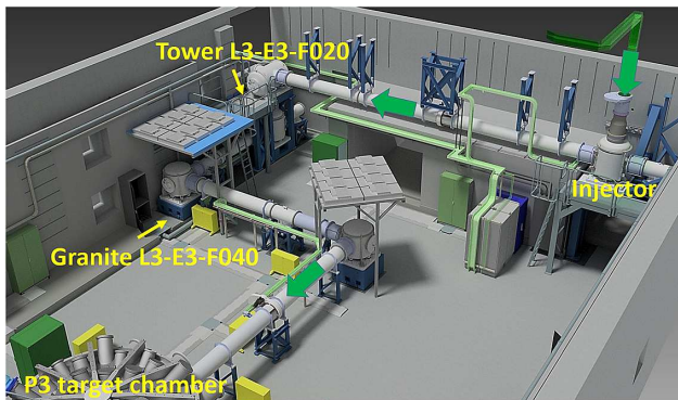
Figure 4. 3D CAD visualization of the HAPLS BT from the injector chamber to the P3 chamber. This figure shows the actual installation in E3.
