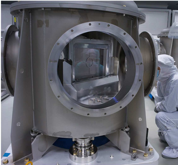
Figure 10. Mounted HAPLS BT mirror installed in its vacuum chamber and both, chamber and breadboard legs/feet bolted onto the aluminium chamber base plate in ISO 5 class cleanroom.
