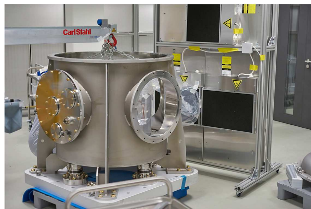
Figure 21. Assembly of HAPLS BT vacuum vessels and optomechanics in cleanroom class ISO 5.
