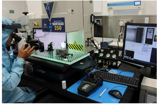
Figure 44. NIF target being assembled at AWE using video coordinate measuring machine supported assembly techniques. (Picture courtesy of AWE.)
