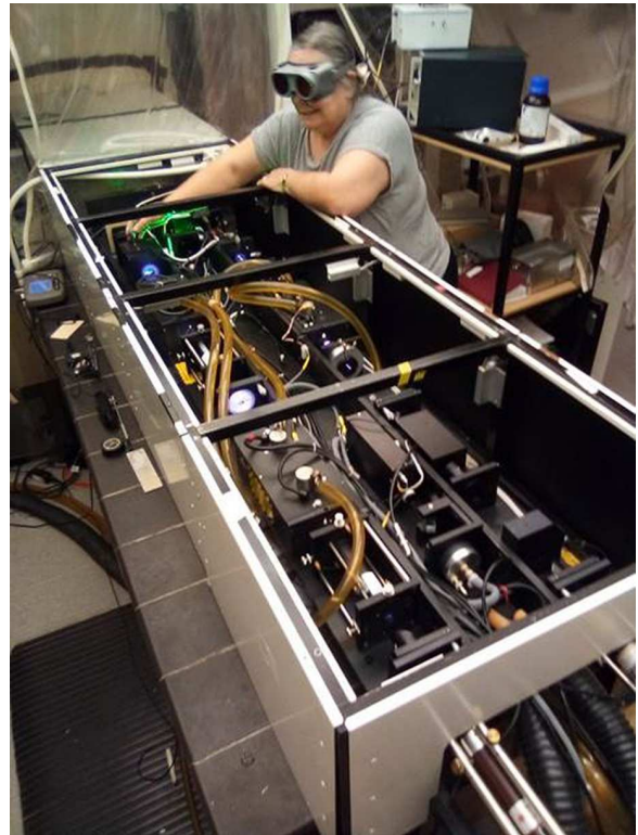
Figure 50. Janet Hull, JEH Lasers, maintaining a JK Lasers Nd:YAG mode locked dye system in 2020 at the Space Geodesy Group, Herstmonceux, East Sussex. Parts of the laser date back to the late 1970s, it was heavily modified in the early 1980s and is still operational.
