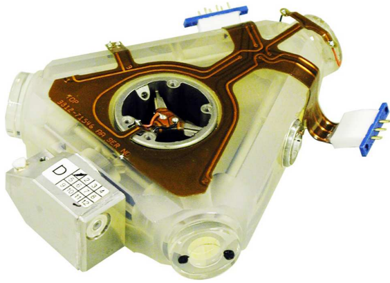
Figure 72. A HeNe laser resonator designed to operate as a ring laser gyro. (Picture courtesy of Leonardo.)
