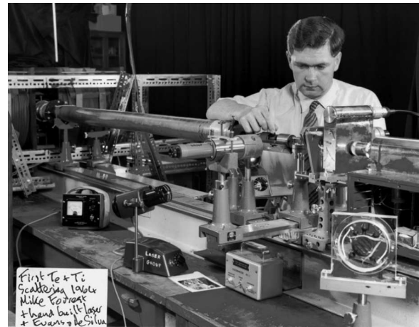
Figure 45. Mike Forrest operates a hand-built laser that is part of a Thomson scattering system used to measure plasma temperatures. This became a major diagnostic technique in the fusion field and is used to this day. (Picture courtesy of Wikipedia.org.)
