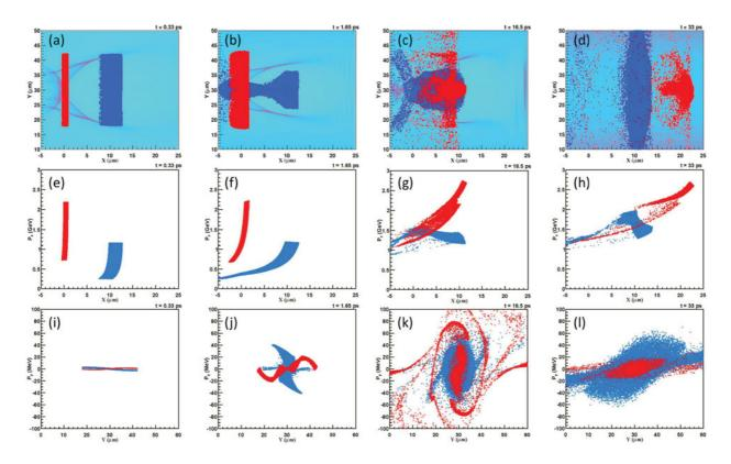
Figure 4. The snapshots of the acceleration processes of forward (red dots) and backward (blue dots) muons from the two-dimensional PIC simulations in Figure 2 at (a) t = 0.33 ps, (b) 1.65 ps, (c) 16.5 ps and (d) 33 ps. (e)–(h) The  $x-p_x$  and (i)–(l)  $y-p_y$  phase spaces of forward (red dots) and backward (blue dots) muons at the four snapshots are also shown, respectively.
