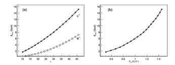
**Figure 5.** The extrapolated relationships of the maximum acceleration energy of muons depending on (a) the bubble's relativistic factor  $\gamma$  and (b) the relevant trapping energy threshold  $E_0$  from the one-dimensional analytic model. The extrapolation of electrons (open circles) in the same parameters is also shown for comparison.
