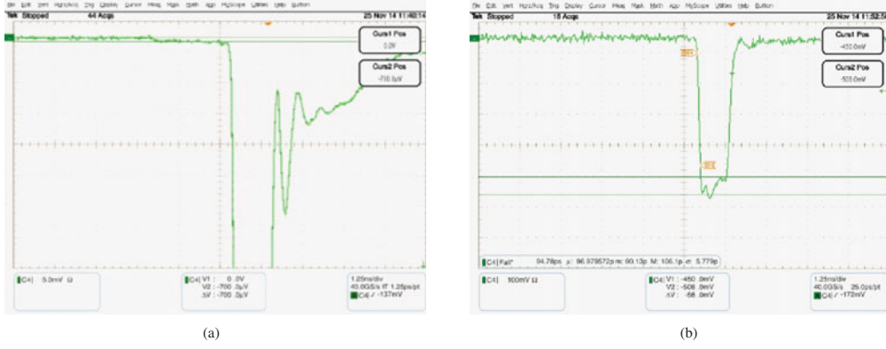
Figure 15. The high contrast temporal waveform (600 : 1). (a) Low amplitude pedestal; (b) high amplitude step.
