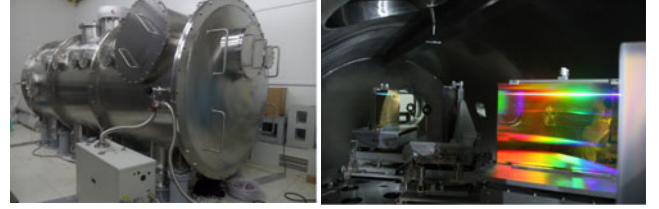
Figure 13. Compressor tank (left) and an inner image of the gold-coated gratings (right).
