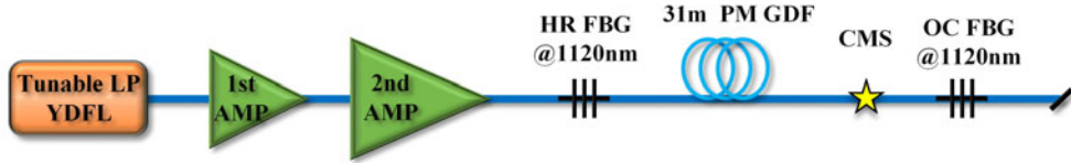
Figure 1. The experimental schematic of the linearly polarized Raman fiber laser. LP: linearly polarized; AMP: amplifier; GDF: germanium-doped fiber; CMS: cladding mode stripper.
