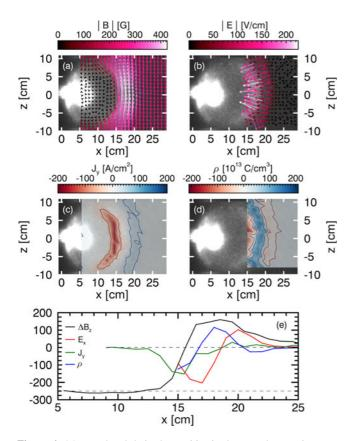
**Figure 6.** Measured and derived quantities in the x-z plane at time  $t = 0.5 \,\mu$ s. (a) Measured vector magnetic field **B**. (b) Vector electric field **E** derived from the gradient of the measured electrostatic potential. (c) *Y*-component of the current density  $J_y$ , derived from the measured magnetic field. (d) Charge density derived from the measured potential. (e) Profiles taken along z = 0 in (a)–(d). Also shown in (a)–(d) is an image of plasma self-emission at the same time.
