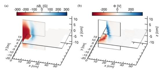
Figure 3. Composite plots of (a) the magnitude of the relative magnetic field  $\Delta B_z = B_z - B_0$  and (b) the electrostatic potential  $\Phi$  in the *x*-*z* and *x*-*y* planes at the same time  $t = 0.5 \,\mu$ s. Each plane is comprised of thousands of separate laser shots, showing a high degree of reproducibility. The target is located at {*x*, *y*, *z*} = {0, 0, 0}.
