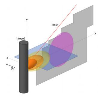
**Figure 1.** Schematic of the experimental setup in the LAPD. A high-repetition-rate laser hits a plastic target embedded in an ambient magnetized plasma. The target rotates and translates in between laser shots. The resulting interaction between the laser plasma and ambient plasma is scanned with magnetic flux ('bdot') probes and emissive Langmuir probes in two intersecting planes, x-z (blue) and x-y (gray). The location of the high-density ambient plasma at z = 0 is shown in purple.
