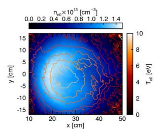
**Figure 2.** Langmuir probe measurements of the initial electron density  $n_{e0}$  and temperature  $T_{e0}$  in the x-y plane. The target is located at  $\{x, y\} = \{0, 0\}$ .
