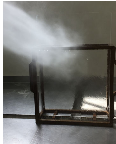
Figure 8. 857 mm × 587 mm amplifier blast shield with ultra-BAC spray cleaned with deionized water.
