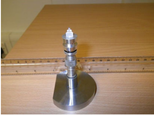
Figure 3. Sample mounted onto X-ray CT holder. The carbon foam is just visible on the top.
