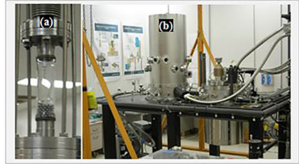
Figure 6. Fluidized bed with a massive of Au/Pd-coated PAMS shells of a 4 mm diameter. (a) Bed is out of the cryostat; (b) bed is inside the cryostat. Bed fluidized at 9 K (taken from Ref. [54]).
