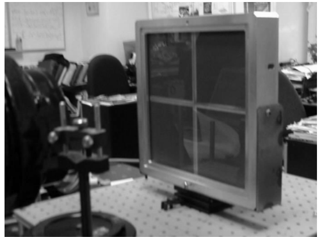
Figure 3. Photo of the bimorph deformable mirror 260 mm \times 260 mm attached in its mounting.
