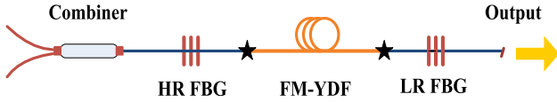
Figure 1. Brief schematic diagram of the 1018 nm fiber laser. HR, high-reflectivity; LR, low-reflectivity; FM-YDF, few-mode Yb-doped fiber.
