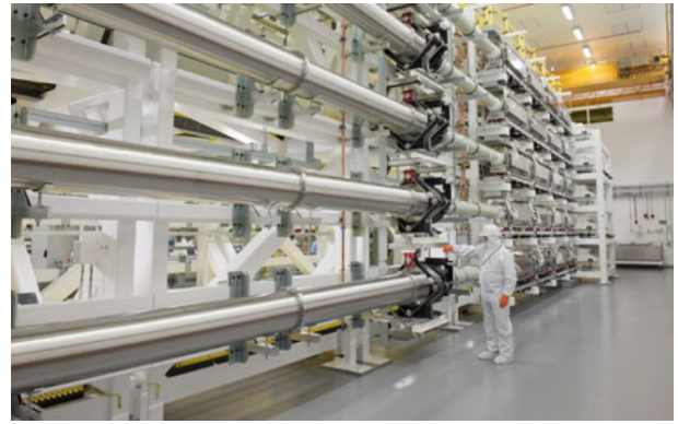
Figure 6. Orion's long pulse amplifier chain.
