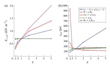
**Figure 7.** The dependence of the saturation value (a) and saturation length (b) on the waveguide and trigger bunch parameters. Here, the index 0 represents the parameter value as in Figure 2 or Ref. [18].
