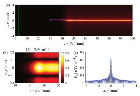
Figure 4. (a) A two-dimensional plot of the longitudinal wake  $|E_z|$ . The green rectangle is the location of the trigger bunch. (b) The same as (a) but in the region that is marked in magenta in (a). (c) The radial dependence of the wake at  $z - \beta ct = 50$  mm.
