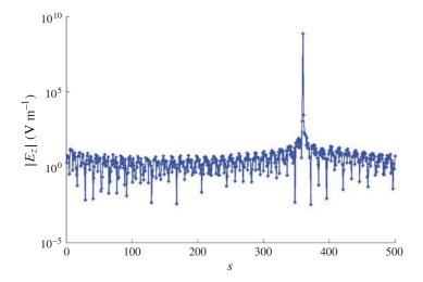
**Figure 3.** The mode spectrum of the wake  $|E_{z,s}(\beta cT = 10 \text{ cm}, r = 0)|$ . Here, the single-resonance mode is s0 = 360.
