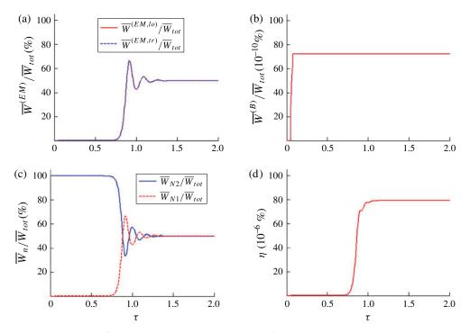
Figure 5. The energy conservation. Here,  $\bar{W}_{N1}$  is the energy of the ground state and  $\bar{W}_{N2}$  is the energy of the excited state; (d) shows the deviation from energy conservation.
