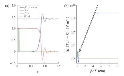
Figure 2. (a) The dynamics of the wake  $\bar{E}_Z(\tau,r=0)$  on the axis (solid curve), the PID,  $\bar{N}$  (dashed–dotted curve), and the trigger bunch profile, f (dashed curve). The value of the saturated wake  $|\bar{E}_{Sat}| = \sqrt{2}$  is shown by the dotted curve. (b) A comparison of the nonlinear wake dynamics in real units (solid curve) with the linear wake dynamics (dots). In addition, the profile of the bunch is drawn as a reference (dashed curve).
