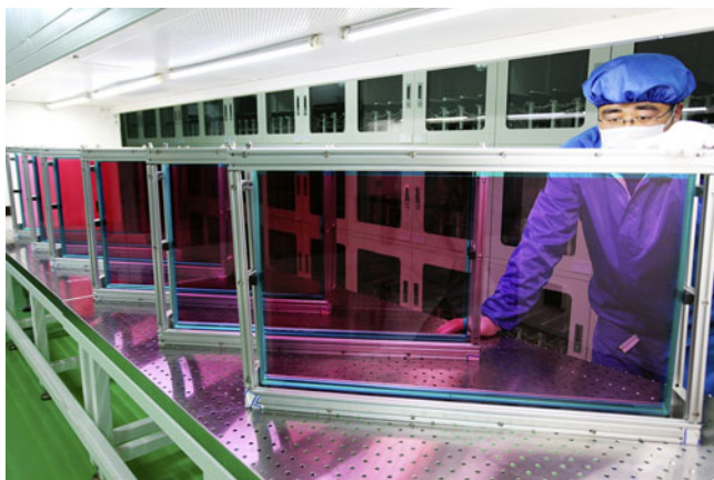
Figure 6. 400 mm aperture N31 glass slabs before installation.
