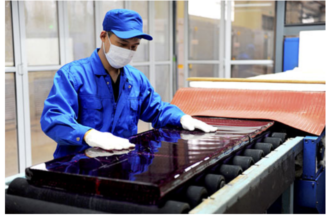
Figure 2. Large size N31 glass running from the annealing Lehr of a continuous melting line.
