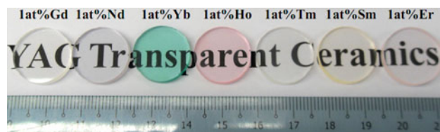
Figure 3. Photograph of different rare-earth doped YAG transparent ceramics fabricated in-house.
