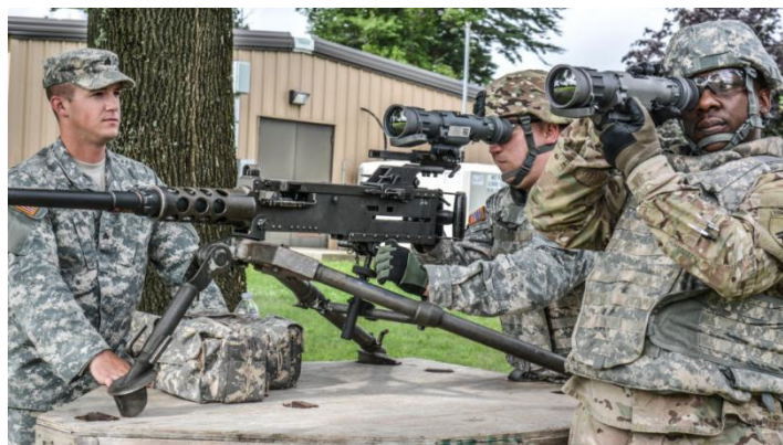
(c) AN/PAS-13E 武器热瞄准镜 (c) AN/PAS-13E thermal weapon sights
