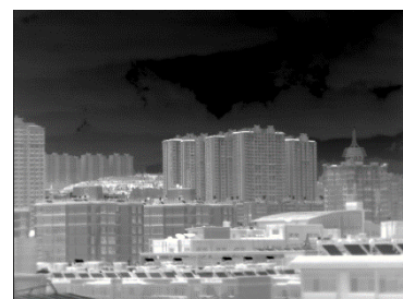
(c) 阈值直方图修正后线性压缩 (平台直方图,阈值为30) (c) Linear compression with modified threshold histogram (platform histogram, threshold of 30)
