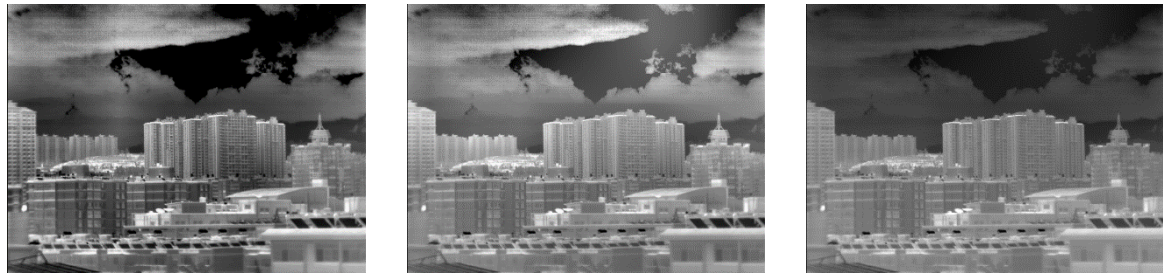
(a) 局部直方图压缩 (b) 基于高斯权重局部直方图压缩 (c) 全局结合局部线性拟合 (a) CLAHE (b) Local histogram compression based on Gaussian weight (c) Global and local linear fitting
