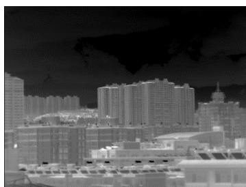
(b) 直方图修正后线性压缩 (b) Linear compression after histogram correction
