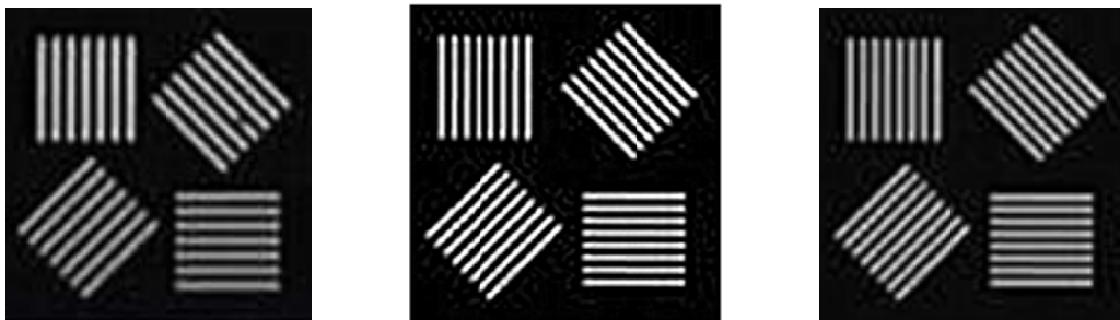
(a) Image of a multi-shot target under -40°C (b) Image of a multi-shot target under -40°C (c) Image of a multi-shot target under 50°C
