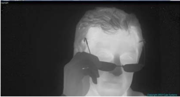
图5 休斯实验室 1\text{ k} \times 2\text{ k}/5\text{ }\mu\text{m} 焦平面在 150 K 下拍摄的照片 Fig.5 Image captured by a 1\text{ k} \times 2\text{ k}/5\text{ }\mu\text{m} MWIR FPA of HRL operated at 150 K
