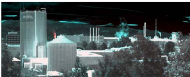
图 14 AIM 384 \times 288 中波双色二类超晶格焦平面成像效果 Fig.14 Bispectral infrared image taken with 384 \times 288 MWIR dual-band T2SL FPA of AIM
