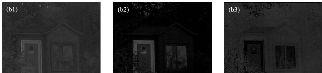
(b1) 绿色植物区域灰度值较大的景深图像 J (b2) 非绿色植物区域灰度值较大的 P'-R' 图像 (b3) 提取出绿色植物区域的景深差分图像 (b1) Depth of field image with large gray value in green plants area (b2) P'-R' image with large gray value in non-green plants area (b3) Depth difference image of green plants area extracted
