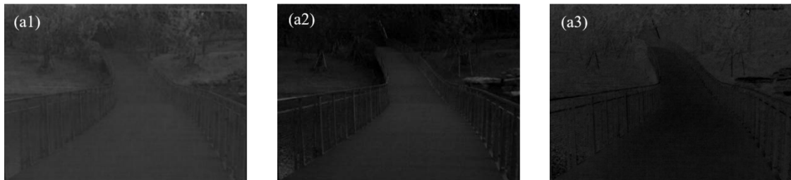
(a1) 绿色植物区域灰度值较大的景深图像 J (a2) 非绿色植物区域灰度值较大的 P'-R' 图像 (a3) 提取出绿色植物区域的景深差分图像 (a1) Depth of field image with large gray value in green plants area (a2) P'-R' image with large gray value in non-green plants area (a3) Depth difference image of green plants area extracted
