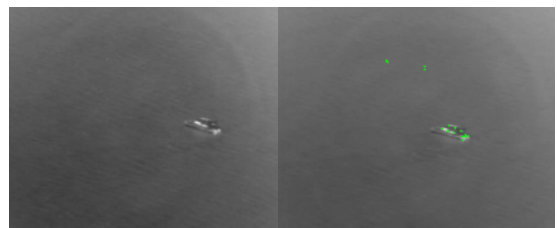
(a) 海面大目标图像 (b) 传统 Harris 角点检测结果 (a) Large sea target image (b) Traditional Harris corner detection results
