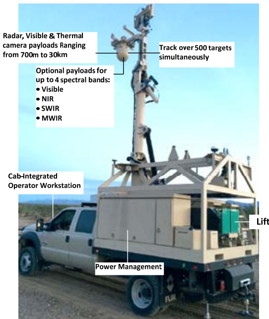
图 8 基于改装皮卡和曲臂式升降机的 FLIR MVSS 光电桅杆 Fig.8 Modified truck and crank arm lift based FLIR MVSS opto-electric mast
