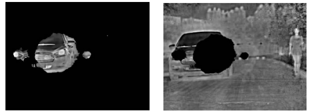
(e) 融合图像晕光区 (f) 融合图像非晕光区 (e) Halo region of fusion image (f) No-halo region of fusion image
