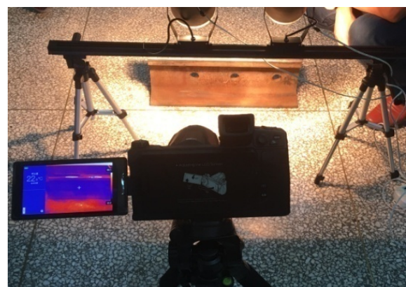
Fig.6 Experimental photo of infrared thermal wave nondestructive testing of rail foot cracks
