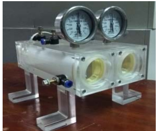
图3 双腔红外气室 Fig.3 Dual-chamber infrared gas chamber
