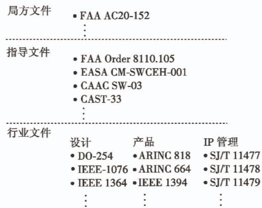
图 2 COTS IP 适航审定文件体系 Fig.2 Airworthiness certification documentations for COTS IP
