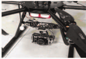
图6 实验用搭载于多旋翼无人飞行器的机载云台 Fig. 6 Airborne platform mounted on multi-rotor UAV for experiment
