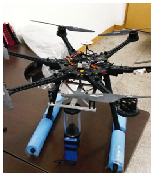
图 5 微型无人机载实时全景成像系统实物 Fig. 5 Material object of UAV real-time panoramic imaging system
