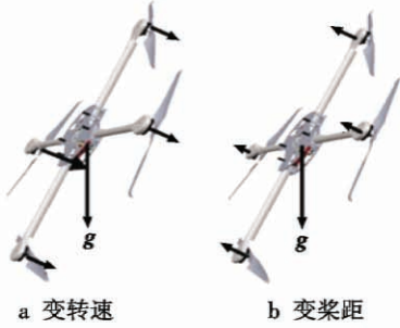
图 1 变转速和变桨距大角度时力响应比较 Fig.1 Force response comparison of variable speed and variable pitch in high angle
