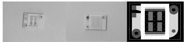
(a)点荧光粉前 (b)点荧光粉后 (c)AC LED结构图
