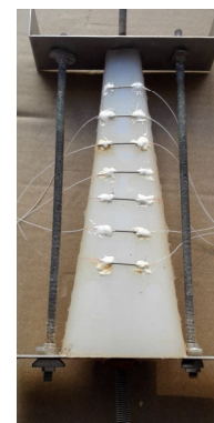
Fig.2 The fixed soft robot finger for calibration: (a) Schematic diagram; (b) Photograph (sensor 1 to 7 named from top to bottom)
