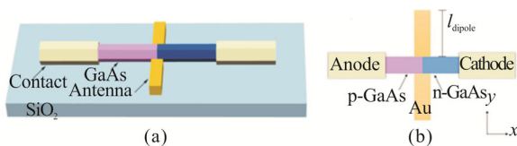
Fig.1 The schematic of the device: (a) Illustration of a contacted axial PN junction GaAs NW with a dipole antenna on its both sides; (b) Top view of the open-sleeve dipole antenna consisting of a dipole antenna
