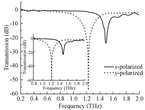
**Fig.2 Transmission spectra corresponding to different polarization waves at the insulation phase of VO<sub>2</sub> (The inset shows the case without VO<sub>2</sub> pads)**
