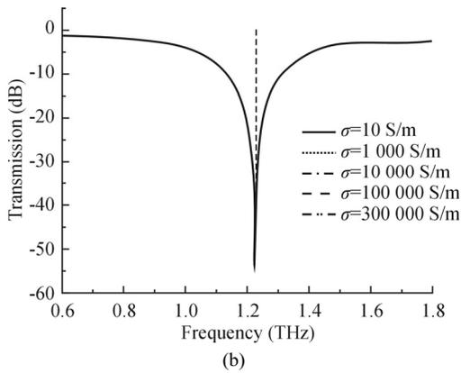
**Fig.3 Simulated transmission spectra for different conductivities of VO<sub>2</sub>: (a) x-polarization THz wave; (b) y-polarization THz wave**
