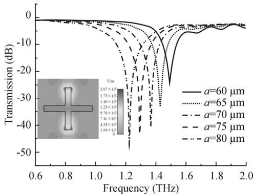
**Fig.4 Transmission spectra of x-polarization THz wave for different y-axis arm lengths (The inset shows the charge accumulation at the edges of the cross-arm.)**
