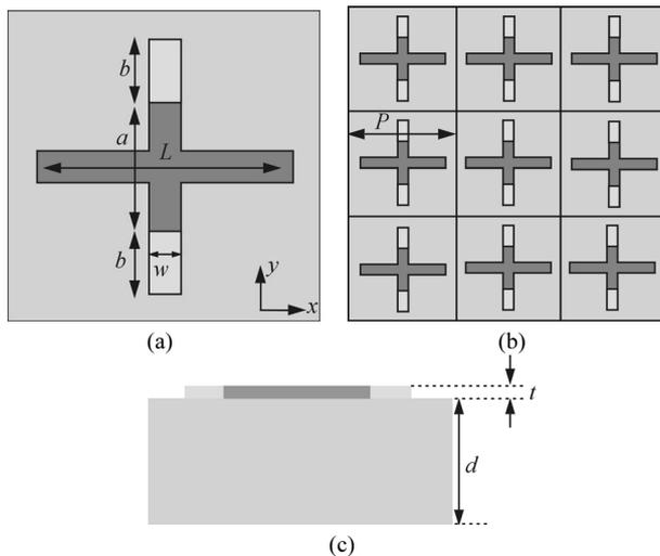
**Fig.1 Schematic structure of the proposed device ( $L=80 \mu\text{m}$ ,  $a=60 \mu\text{m}$ ,  $b=10 \mu\text{m}$ ,  $w=10 \mu\text{m}$ ,  $P=100 \mu\text{m}$ ,  $t=1 \mu\text{m}$ ,  $d=500 \mu\text{m}$ ): (a) Geometry of the unit cell; (b) The period structure; (c) Side view of a single unit cell**
