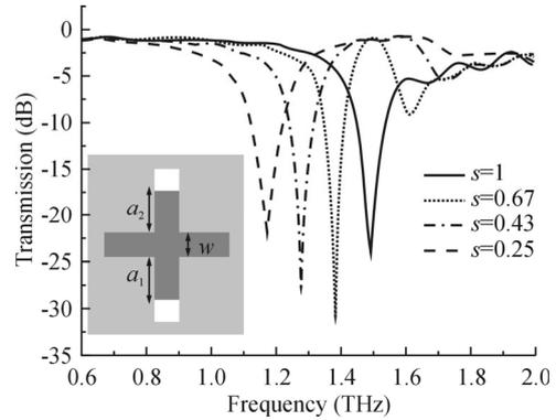
**Fig.5 Transmission spectra of x-polarization THz wave for different asymmetric factors**
