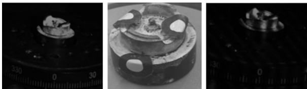
(a) The proposed method (b) The sticking marked point method (c) Projected fringe patterns of cam
