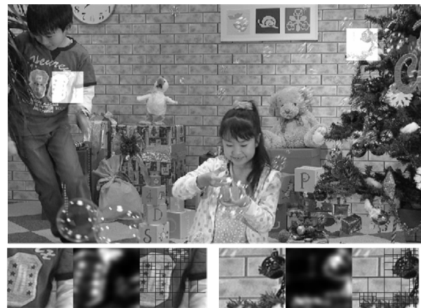
Fig.3 The saliency map and partitioning result in LCUs for sequence “Blowing Bubbles”
