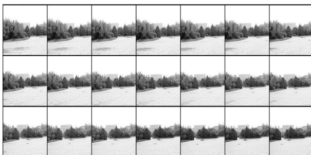
Fig.8 Elemental images captured by the outdoor integral imaging system
