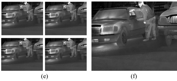
Fig.4 (a) A gathered LRI; (b) The image reconstructed by bicubic interpolation; (c) The set including the LRIs of the first generation; (d) The image reconstructed by LRIs from (c) using traditional regularized SRR; (e) The set including the optimal LRIs of the final generation; (f) The image processed by the proposed algorithm, which is reconstructed by the optimal LRIs from (e)
