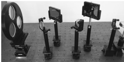
Fig.5 The experimental setup of the long-distance optical signal 3-aperture diversity reception system
