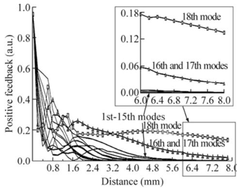
**Fig.5 The positive feedback of each supermode at the output end considering the self-coupling where  $D_1$  and  $D_2$  are adjusted together**
