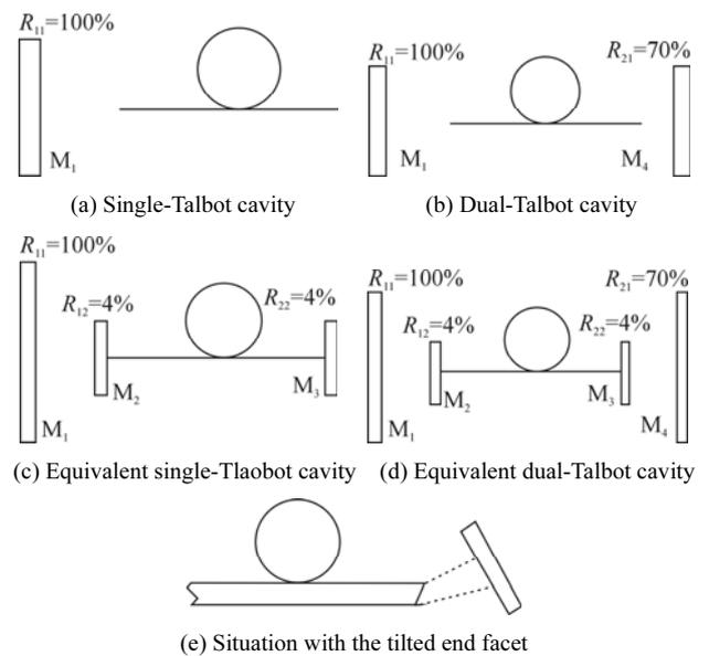
**Fig.4 Schematic diagrams and the corresponding equivalent schematic diagrams of the single-Talbot cavity and the dual-Talbot cavity**
