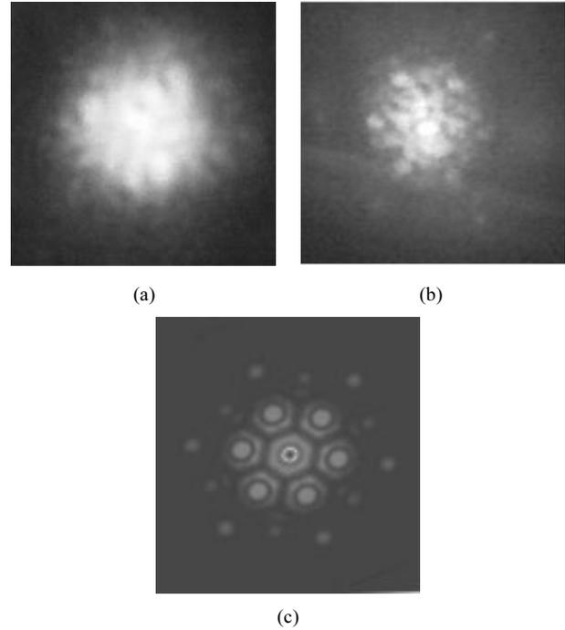
**Fig.6 The comparison of the experiment results of the output obtained in (a) the single-Talbot and (b) dual-Talbot cavities; (c) Far-field calculation result of the 18th mode**
