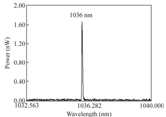
**Fig.7 Output spectrum of the multi-core PCF based on dual-Talbot cavity**
