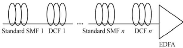
Fig.3 Schematic diagram of the transmission link
