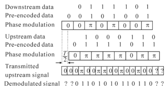
Fig.1 Operating principle of time interleaved phase remodulation
