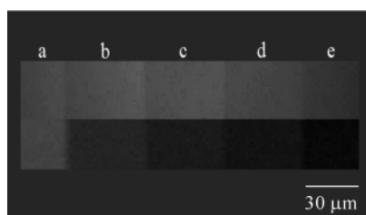
Fig.4 Mapping information of Raman spectra of In-In 2 O 3 grayscale film with five different gray levels (a-e)
