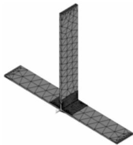
Fig.2 FE model and mesh of \pi -joint
