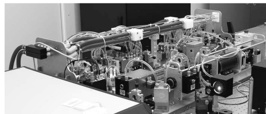
Fig. 7 The Advanced LIGO 200 W laser under assembly
