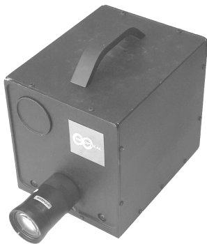
图 3 基于带通滤光片的多光谱成像系统 Fig. 3 Multi-spectrum imaging system with band-pass filters
