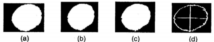
Fig. 4 (a) Original NF image, (b) the image after the median filter, (c) the image after thresholding, and (d) the final image.
