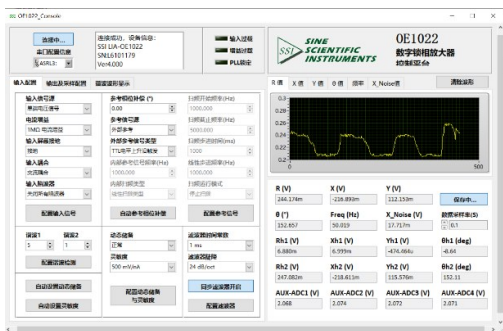
图 18 锁相放大器显示的太赫兹探测响应波形 Fig. 18 Terahertz detection waveform displayed by a phase-locked amplifier
