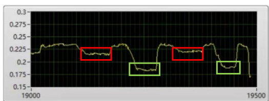
图 19 对不同隔挡物(A4纸和铜板)的透射结果 Fig. 19 Transmission results for different barriers (A4 paper and copper sheet)
