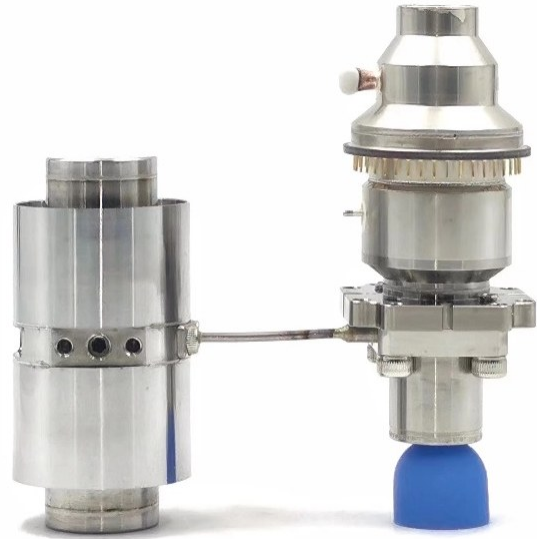
Fig. 1 The photograph of the MWIR HgCdTe HOT IDCA 图1 碲镉汞中波高温组件实物图
