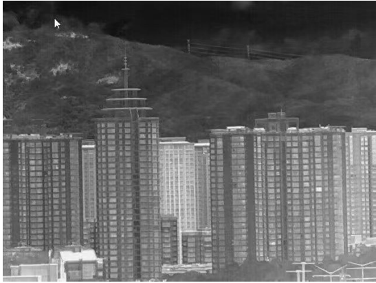
Fig. 9 The IR-image at an operating temperature of 150 K from MWIR HgCdTe HOT FPAs
